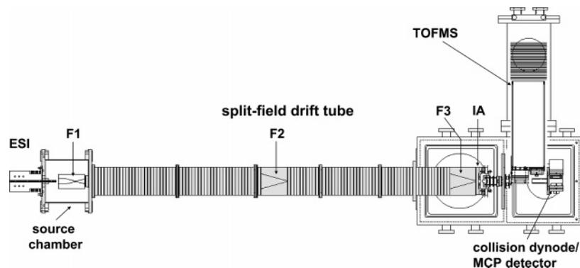
**Figure 1.** Schematic diagram of the IMS-MS instrument used in the current studies.
